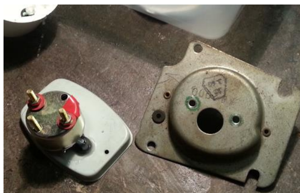
Air core meter fixed to faceplate with araldite
