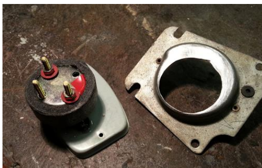
Foam around air core meter
